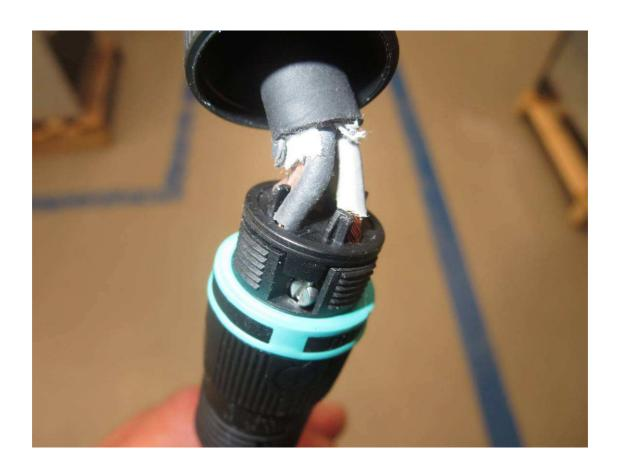
Figure 6 inspection after second characteristic numeral 6
