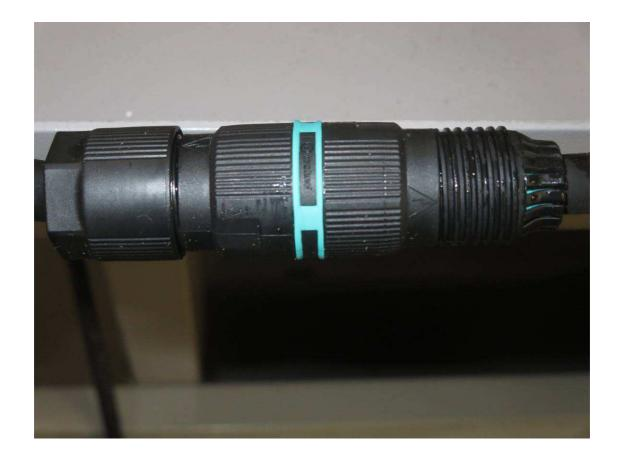
Figure 5 inspection after second characteristic numeral 6
